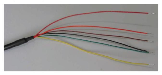
• Connect the red and black wire to the asset power source. If the asset is installed on a trailer then the connection will be to the back light that is powered when the trailer is connected to the tractor.
